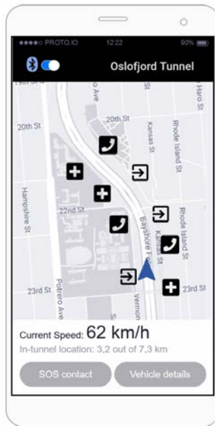
Figure 15: A UI prototype of the RiskTUN BLE mobile application for a vehicle inside the tunnel.
